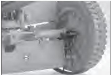
3. Unfold the gun support legs and insert the fixing pin;
